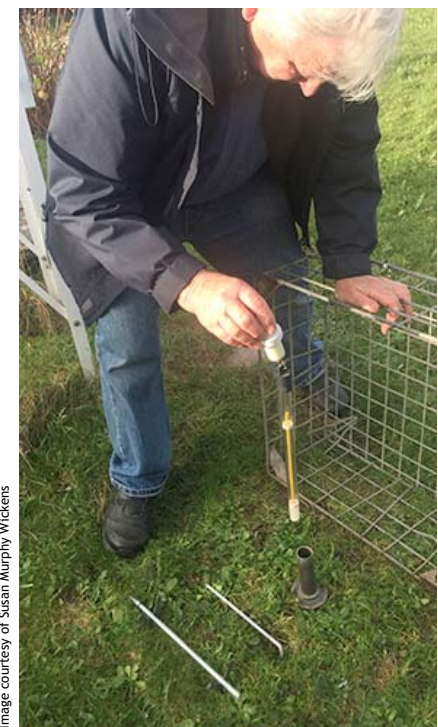
Checking the temperature 30 cm below ground level.
